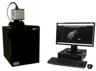
The *FluorVivo family* represents **the next generation** of *in vivo* fluorescence imaging of small animals. For situations where a monochrome camera is the preferred choice, INDEC BioSystems now offers the FluorVivo 1000, a complete, turn-key, in vivo imaging system, based on monochrome camera and filter wheel technologies.
